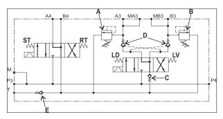
Figure 7-13. Secondary Manifold Schematic
