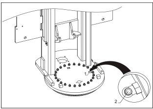
Figure 5-3. Swing Bearing Race Lubrication
