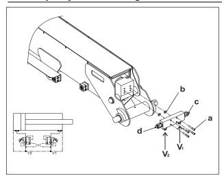
Figure 7-18. Telescope Cylinder Holding Valve - Removal/Installation
