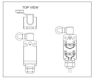
Figure 8-8. Actuators Setting
