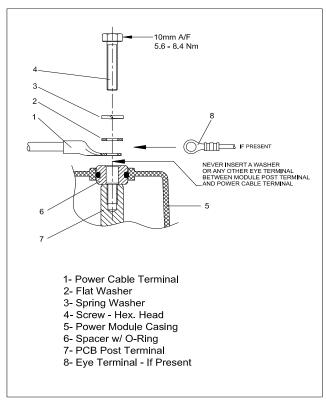
Figure 8-24. Cables on Power Module Post Terminal
