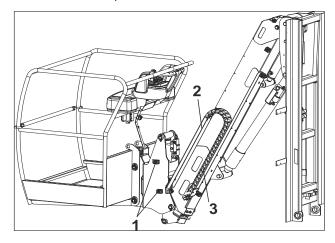
Figure 6-2. Platform Support and Slave Cylinder Removal - 1 of 4
