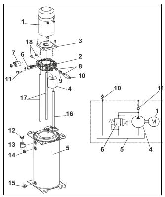
Figure 7-2. Hydraulic Power Unit
