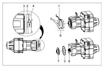
Figure 4-2. Brake Disassembly
