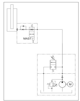
Figure 3-3. Mast Lift System - Basic Schematic
