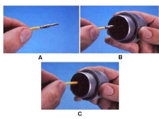
Figure 11-14. HD/HDP Contact Installation
