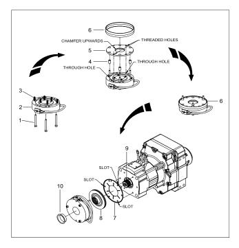
Figure 4-4. Brake Assembly
