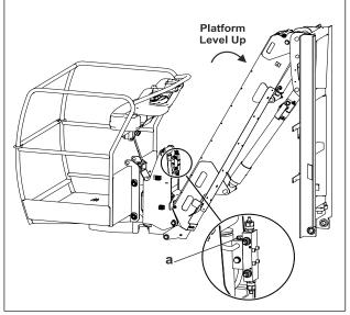
Figure 7-22. Air Bleeding From Piston Side
