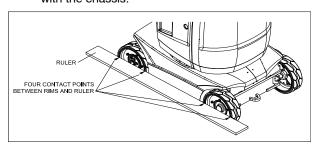
Figure 9-5. Wheel Straightening
