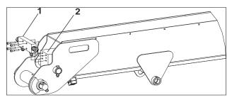
Figure 6-9. Telescope and Cylinder Removal - 1of 5
