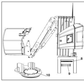
Figure 5-10. Swing Bearing Removal - 6 of 6
