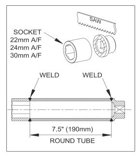
Figure 5-20. Long Hollow Body Socket
