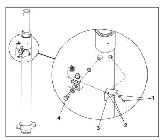
Figure 7-14. Mast Cylinder Holding Valve
