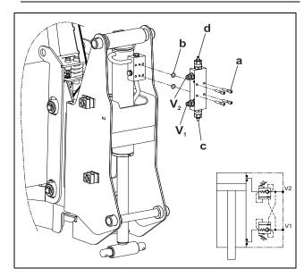
Figure 7-19. Slave Cylinder Holding Valve
