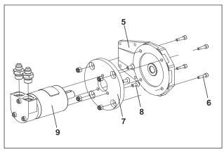
Figure 5-14. Swing Drive Disassembly - 2 of 3
