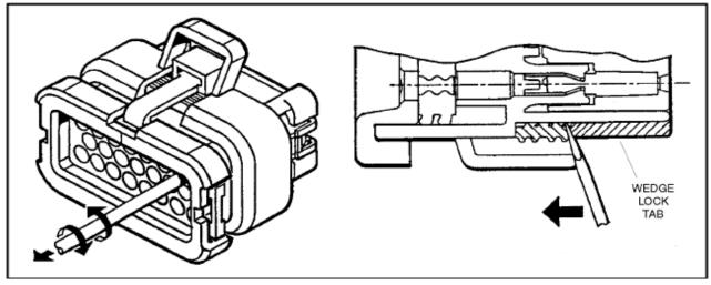
Figure 11-10. Connector Disassembly
