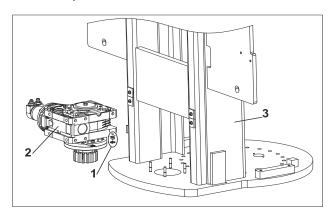
Figure 5-12. Swing Drive Removal
