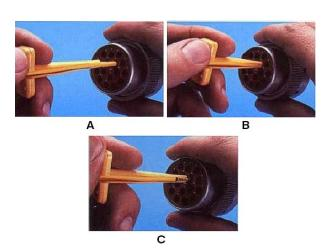
Figure 11-16. HD/HDP Contact Removal
