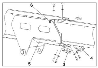
Figure 6-10. Telescope and Cylinder Removal - 2 of 5
