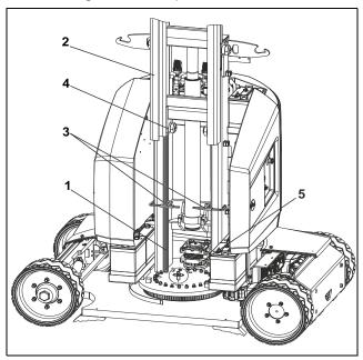
Figure 5-39. Mast Cylinder Removal - 2 of 8
