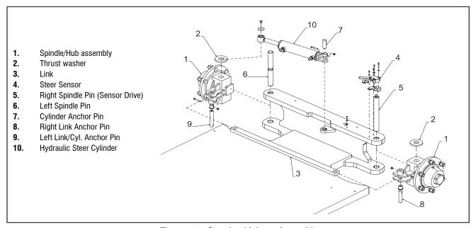
Figure 4-9. Steering Linkage Assembly
