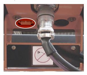
Figure 9-2. Hand Held Analyzer Connection
