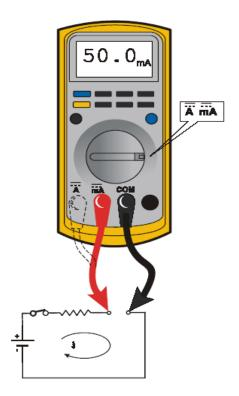
Figure 11-4. Current Measurement (DC)
