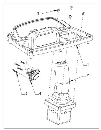
Figure 8-30. Joystick Controls - Installation
