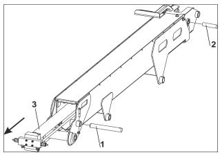
Figure 6-14. Telescope and Cylinder Removal - 1 of 3
