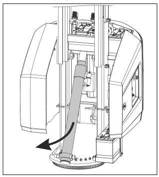
Figure 5-45. Mast Cylinder Removal - 8 of 8
