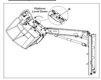
Figure 7-21. Air Bleeding From Rod Side
