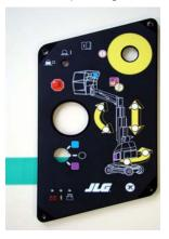
Re-install the components on the panel, re-connect the connectors on the PCB and re-install the panel assembly.
