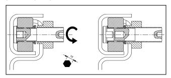
Figure 5-17. Roller Removal
