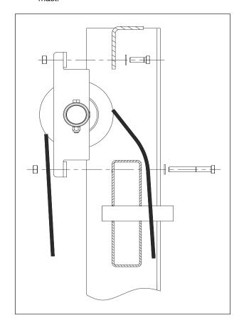
Figure 5-37. Pulley Support Removal
