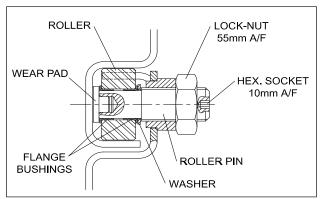
Figure 5-16. Roller Assembly
