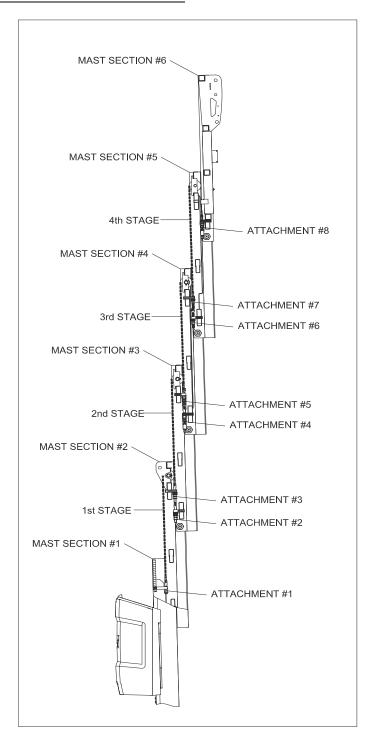
Figure 5-24. Chains Stages and Attachments Description
