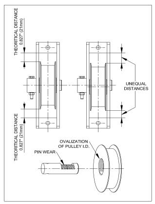
Figure 5-36. Pulley Assembly Wear
