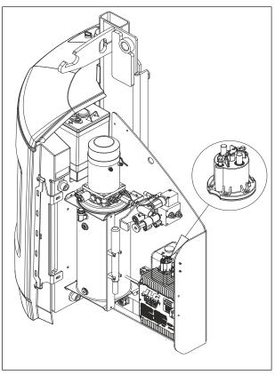
Figure 8-5. Main Power Contactor Relay
