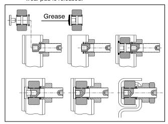
Figure 5-18. Roller Installation
