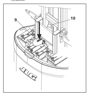
Figure 5-42. Mast Cylinder Removal - 5 of 8
