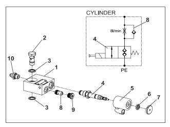
Figure 7-17. Jib Cylinder Holding Valve - Schematic/Exploded View
