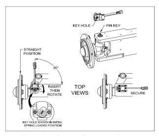
Figure 4-10. Steering Sensor Installation
