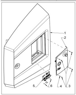
Figure 8-28. Ground Control Box Circuit Board - Installation
