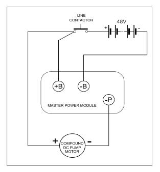
Figure 3-2. Hydraulic Pump Electric Schematic
