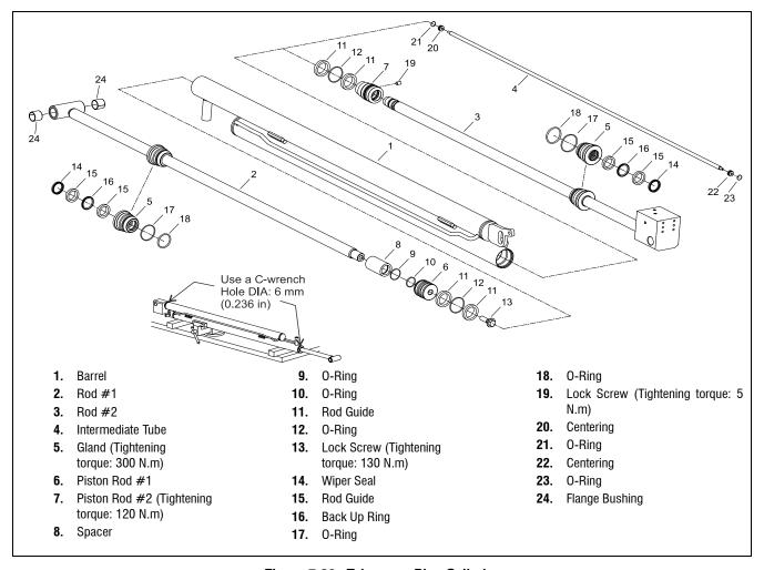
Figure 7-30. Telescope Plus Cylinder
