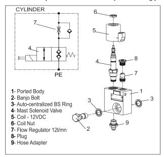
Figure 7-15. Mast Cylinder Holding Valve - Schematic/Exploded View
