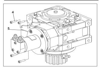
Figure 5-13. Swing Drive Disassembly - 1 of 3
