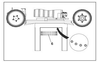
Figure 5-7. Swing Bearing Removal - 3 of 6
