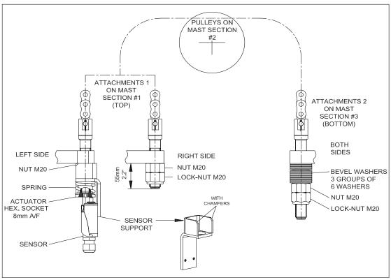
Figure 5-25. First Chain Stage
