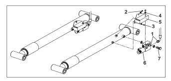
Figure 7-16. Jib Cylinder Holding Valve - Removal/Installation
