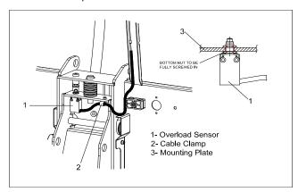
Figure 8-13. Overload Sensor
