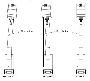
Figure 5-19. Mast Sections Vertical Alignment
