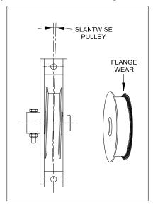
Figure 5-35. Slantwise Pulley
