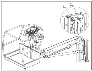
Figure 8-9. Jib Elevation Limit Switches
