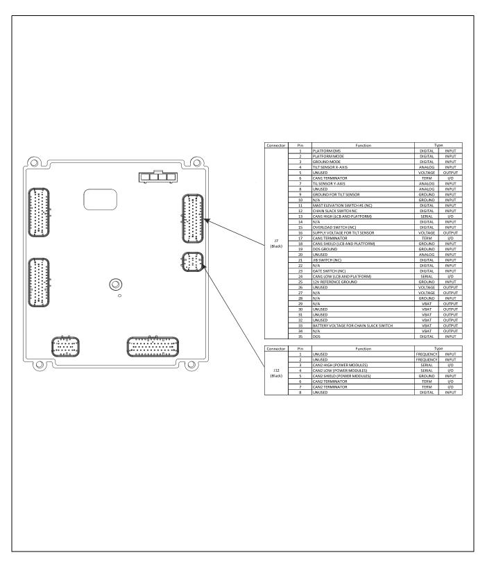
Figure 8-26. Ground Control Station Connectors - 2 of 3
