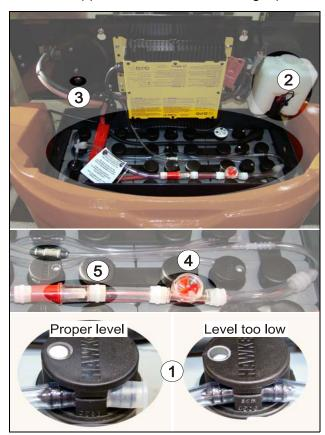
Figure 8-2. Battery filling
