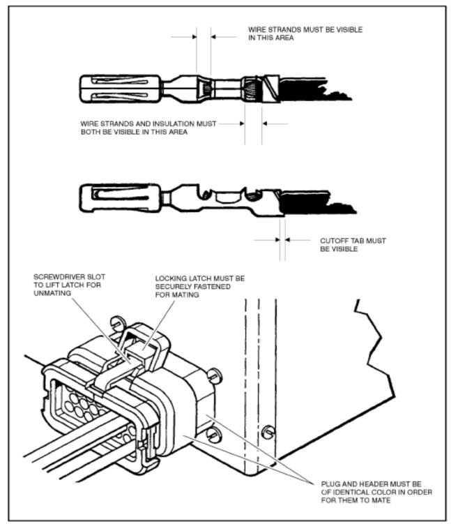
Figure 11-11. Connector Installation
