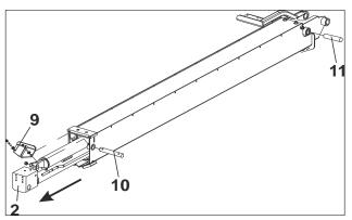
Figure 6-12. Telescope and Cylinder Removal - 4 of 5
