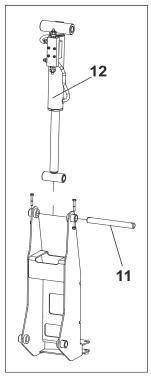
Figure 6-6. Platform Support and Slave Cylinder Removal - 4 of 4
