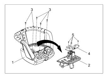
Figure 8-29. Upper Control Box Circuit Board - Installation
