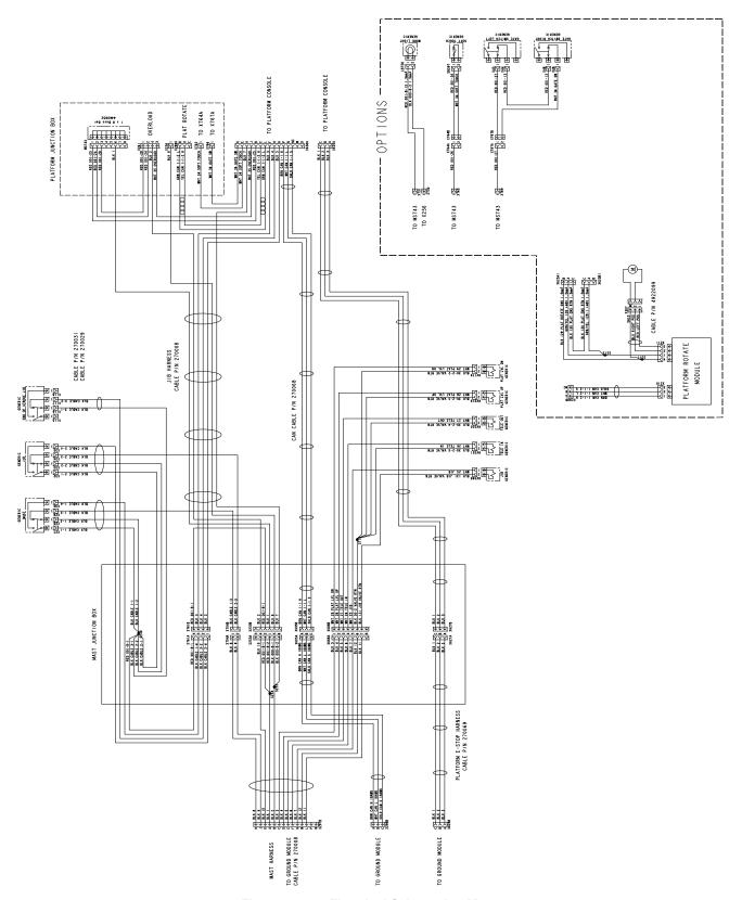
Figure 11-24. Electrical Schematic - Mast
