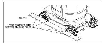
Figure 8-18. Wheel Straightening
