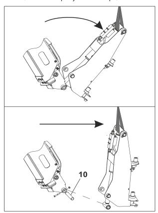
Figure 6-5. Platform Support and Slave Cylinder Removal - 3 of 4
