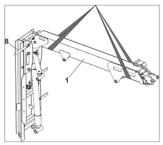
Figure 6-8. Boom and Cylinder Removal - 2 of 2
