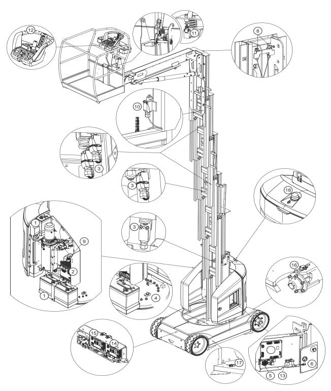
Figure 8-1. Control Components Location
