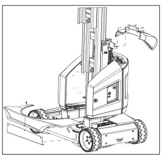
Figure 5-38. Mast Cylinder Removal - 1 of 8
