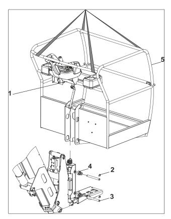
Figure 6-1. Platform Removal-Installation
