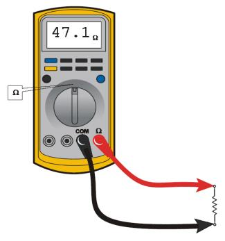
Figure 11-2. Resistance Measurement
