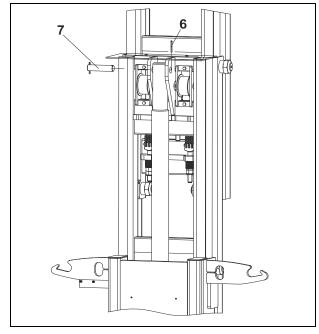
Figure 5-40. Mast Cylinder Removal - 3 of 8
