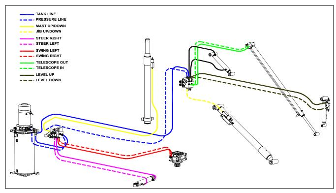
Figure 7-1. Hydraulic Lines Connections
