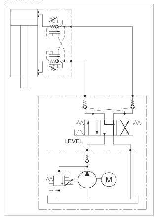
Figure 3-8. Platform Level System - Basic Schematic
