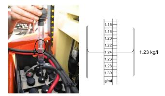
Figure 8-4. Measuring Electrolyte Specific Gravity
