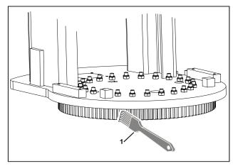
Figure 5-4. Swing Bearing Teeth Lubrication
