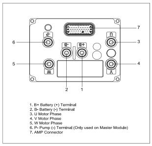
Figure 8-23. Power Module Terminals
