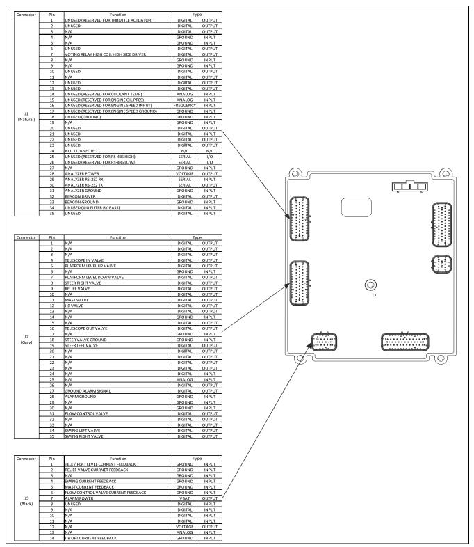
Figure 8-25. Ground Control Station Connectors - 1 of 3
