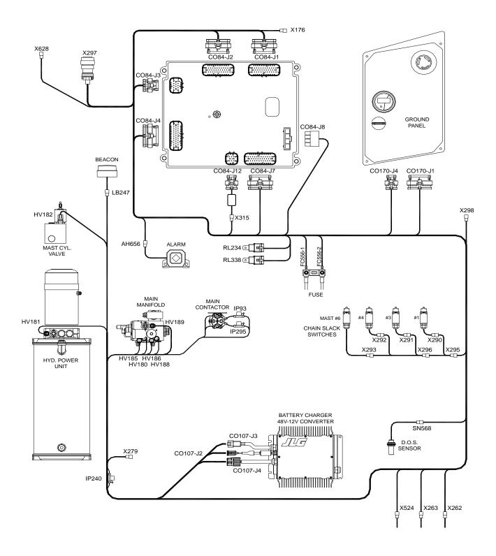
Figure 11-19. Wiring Harness and Connectors - Sheet 2 of 3
