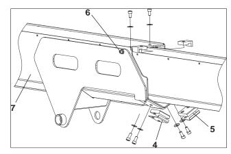
Figure 6-15. Telescope and Cylinder Removal - 2 of 3
