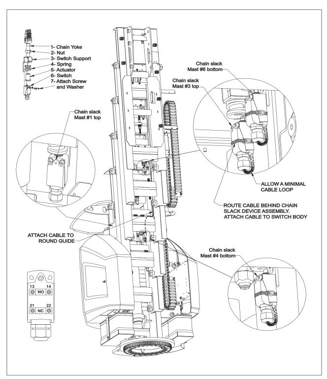
Figure 8-12. Chain Slack Sensors
