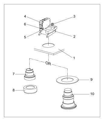
Figure 8-31. Enable/Emergency Stop Switches - Installation
