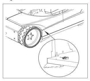
Figure 8-19. Tilt Sensor
