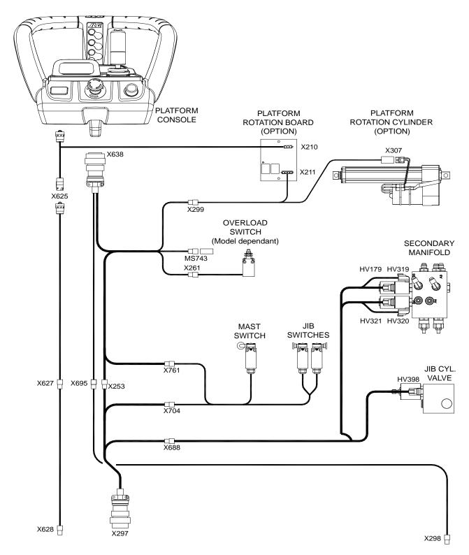
Figure 11-18. Wiring Harness and Connectors - Sheet 1 of 3
