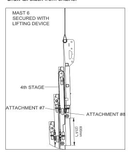
Figure 5-32. Fourth Chains Stage Removal
