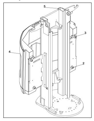
Figure 5-47. Counterweight Removal - 2 of 2
