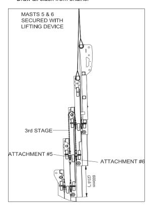
Figure 5-31. Third Chains Stage Removal
