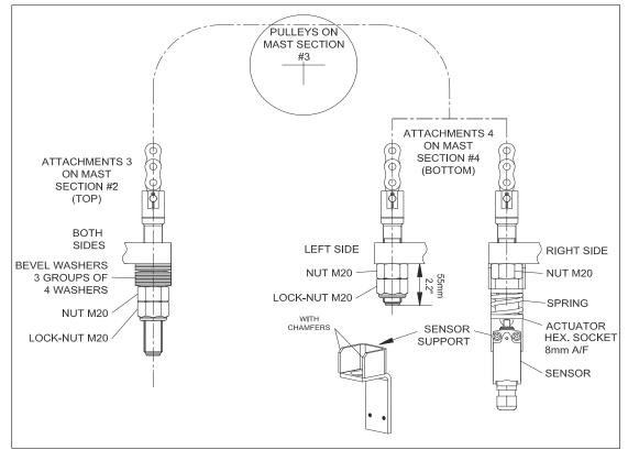
Figure 5-26. Second Chain Stage
