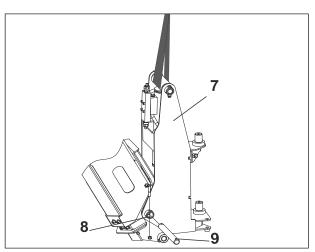
Figure 6-4. Platform Support and Slave Cylinder Removal - 2 of 4
