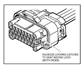
Figure 11-8. Connector Assembly Figure 3
