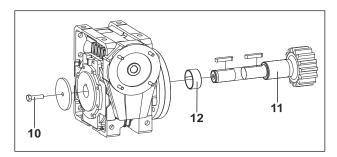
Figure 5-15. Swing Drive Disassembly - 3 of 3
