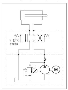
Figure 3-6. Steer System - Basic Schematic
