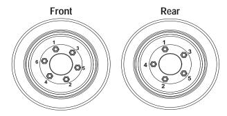
Figure 4-8. Wheel Lug Nut Tightening Sequence
