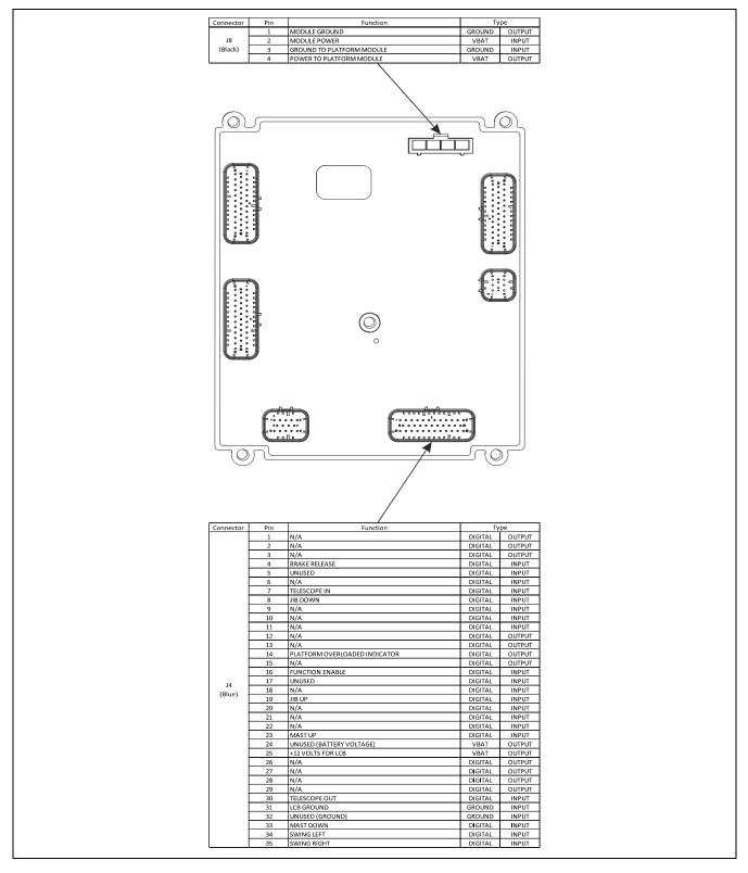
Figure 8-27. Ground Control Station Connectors - 3 of 3
