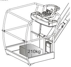
Figure 8-14. Overload Sensor Calibration
