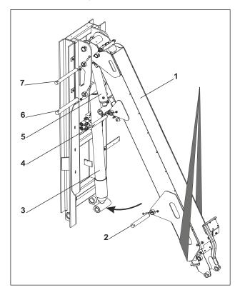
Figure 6-7. Boom and Cylinder Removal - 1 of 2
