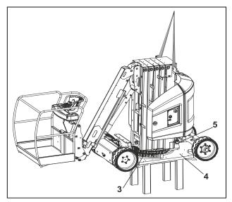
Figure 5-6. Swing Bearing Removal - 2 of 6
