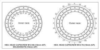
Figure 5-2. Torque Sequence Diagram
