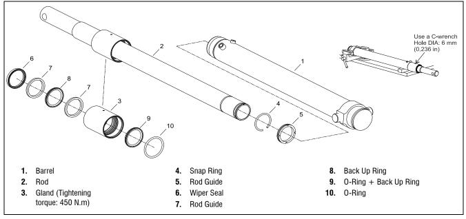
Figure 7-28. Mast Cylinder
