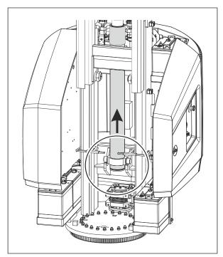
Figure 5-44. Mast Cylinder Removal - 7 of 8
