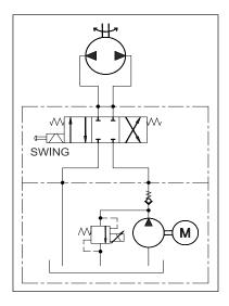
Figure 3-5. Swing System - Basic Schematic
