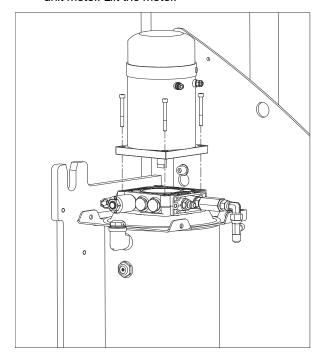
Figure 7-5. Moving Hydraulic Power Unit Motor
