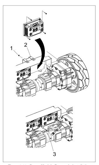
Figure 8-22. Power Module Removal - Installation
