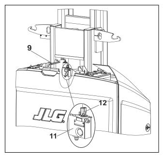
Figure 5-43. Mast Cylinder Removal - 6 of 8
