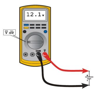
Figure 11-1. Voltage Measurement (DC)
