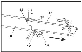
Figure 6-13. Telescope and Cylinder Removal - 5 of 5
