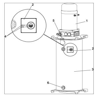
Figure 7-7. Hydraulic Oil Check
