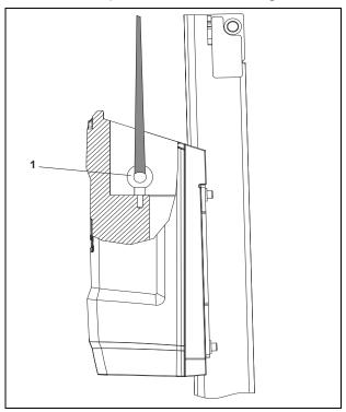
Figure 5-46. Counterweight Removal - 1 of 2
