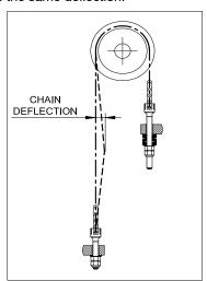
Figure 5-34. Chains Tension Control
