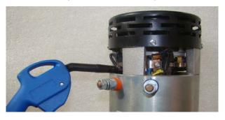
Figure 7-4. Dust Cleaning
