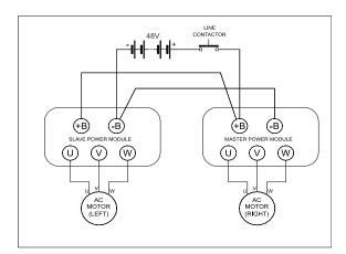
Figure 3-1. Drive Motor Schematic
