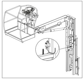
Figure 8-7. Mast Elevation Limit Switches
