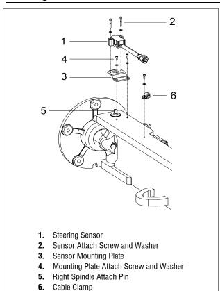
Figure 8-17. Steering Sensor
