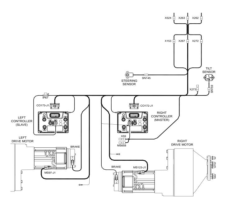
Figure 11-20. Wiring harness and Connectors - Sheet 3 of 3
