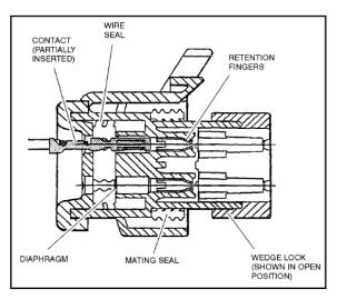
Figure 11-5. Connector Assembly Figure 1
