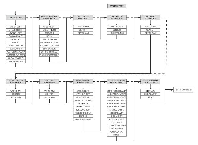
Figure 9-6. System Test Flow Chart
