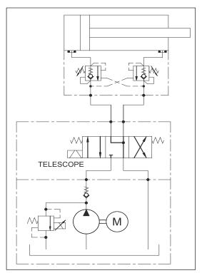
Figure 3-7. Telescope System - Basic Schematic
