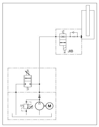
Figure 3-4. Jib Lift System - Basic Schematic
