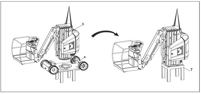
Figure 5-8. Swing Bearing Removal - 4 of 6
