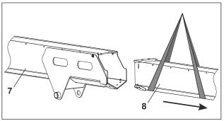
Figure 6-16. Telescope and Cylinder Removal - 3 of 3
