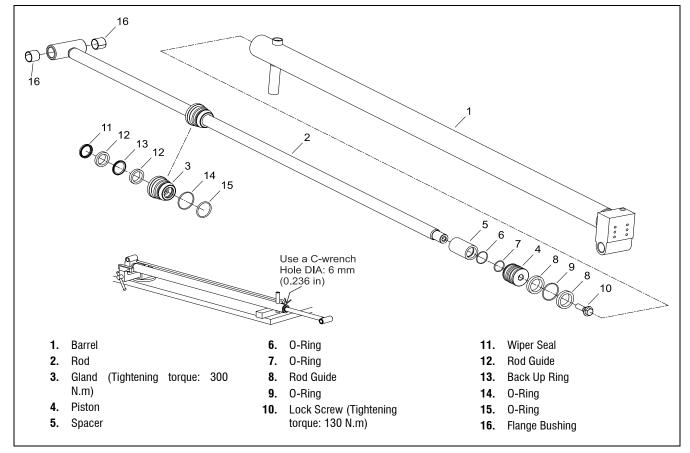
Figure 7-29. Telescope Cylinder
